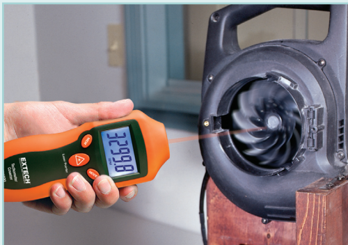
Non-contact fan blade RPM or REV testing
